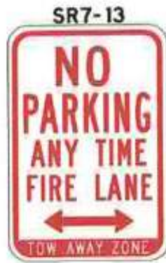
FIGURE 503.3. FIRE LANE SIGNS
